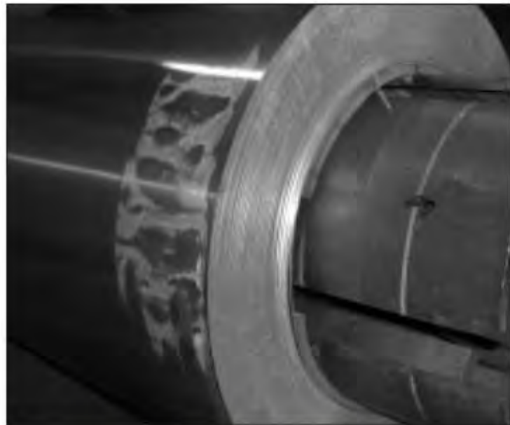
Figure 1 – Water Stain on Coil
